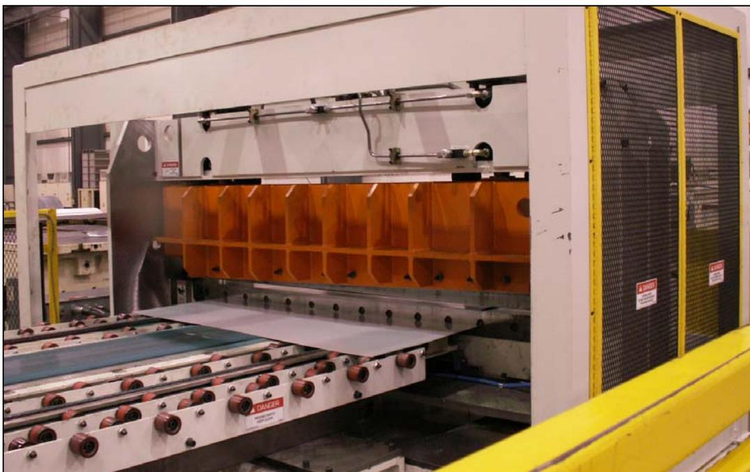
Photo of Servo Driven Oscillating Shear
