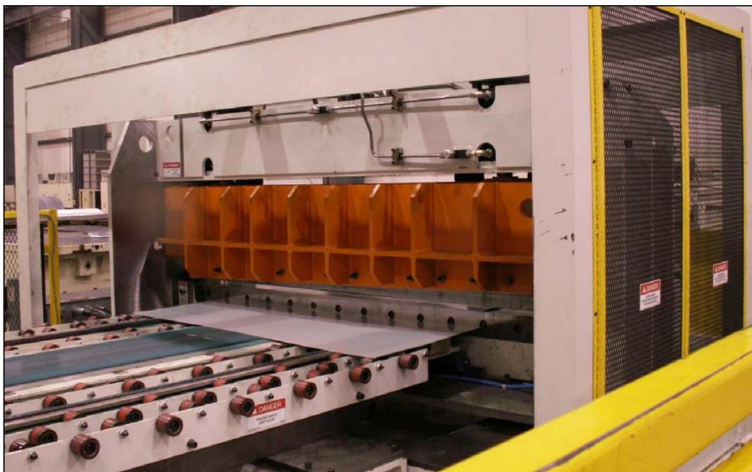
Photo of Servo Driven Oscillating Shear
